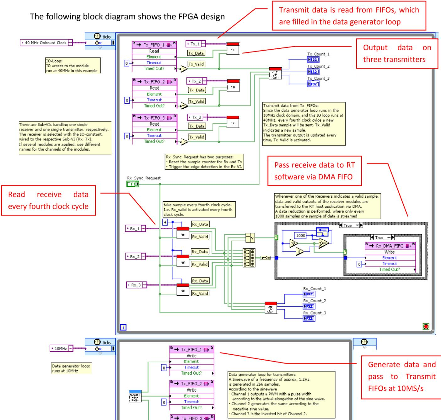
The Tx and Rx Sub-VIs may be used by any user application for reading and transmitting data at different data rates. Note that this is just an example, where FIFO overflow or underflow is not handled. The example has to be adapted to the user's requirements.
