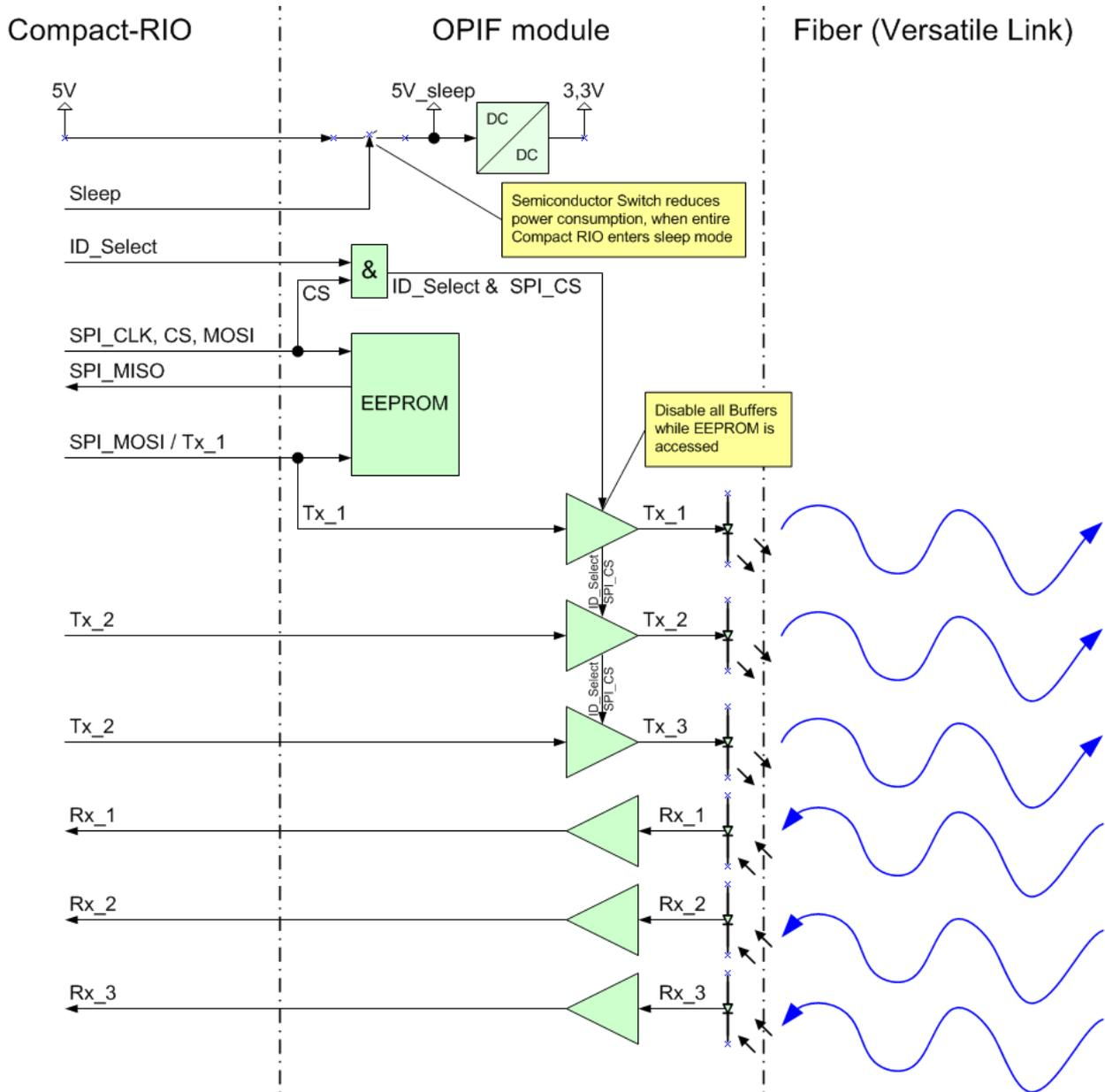
During **start-up or reset** of the Compact-RIO system the IOs between the optical interface module and the Compact-RIO are floating. The module is designed in this way, that the transmitter outputs do not emit light. I.e. **NO LIGHT** should be regarded as the **SAVE STATE**.
