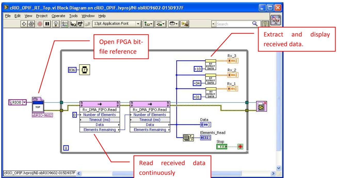
In the RT software the reference to the FPGA-bit-file is opened. With a period of about 836ms the entire received data of approx. one sine wave period is read from the DMA FIFO. Received data bytes contain the bit-streams of all three receiver channels, which are extracted by the bitmasks ("0x01", "0x04", "0x10"). Take care in the RT software that the reference to the FPGA bit-file is a valid path to your bit-file on hard disk.
