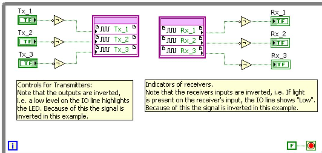
The FPGA IO nodes have to be specified in the project as shown in the following figure:
