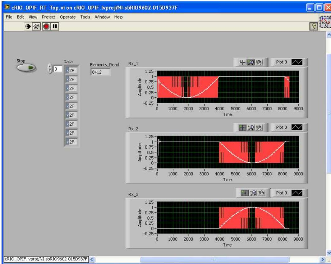
After the VI has started, both RT and the FPGA will automatically run and will generate data. If the optical transmitters and receivers are interconnected, the received data will be displayed as in the figure above.
